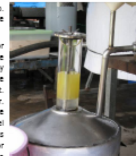
Figure 9: The oil has just risen to the top of the tank and because oil is less dense than water it floats. The oil is siphoned off and weighed to be recorded.
